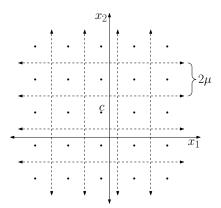
Fig. 1. Illustration of the quantizer for the two-dimensional state space, N=5. The dashed lines define the boundaries of the quantization regions. The black dots define where the quantizer estimates the state to be, given the index of the quantization region that currently contains the state. Note that the quantizer output gives a displacement from  $\boldsymbol{c}$ .
