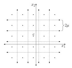
**Fig. 1.** Illustration of the quantizer for the two-dimensional output subspace, N=5. The dashed lines define the boundaries of the quantization regions. The black dots define where the quantizer estimates the projection of the state to be, given the index of the quantization region that currently contains the projection.
